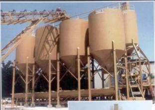
Hamilton Concrete Products Co, of Chattanooga, Tennessee operates this plant. It produces many colors of architectural block, utilizing any number of exotic aggregates. These round sides are easily cleaned between runs of different aggregates. This live bottom batcher both weighs and conveys the material collected from these silos.
