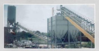
The Paver Systems plant in Lithonia, Georgia was designed and built to supply four aggregates and two cements to two mixers feeding multicolored zero slump concrete to two different paver machines. All storage bins and silos are self-cleaning.
